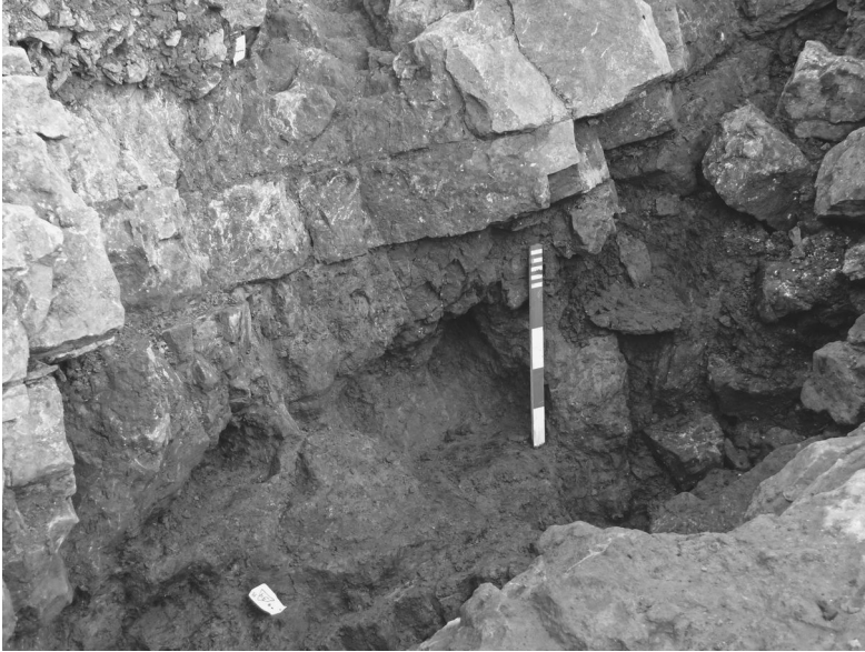
Fig. 6.18. Drift extraction of bedded copper mineralization at The Lumb, Ecton mine, Staffordshire
