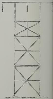
Types of towers—The tall tower is standard, 82 feet high; the smaller is a snow-tower, 49 feet in height.
