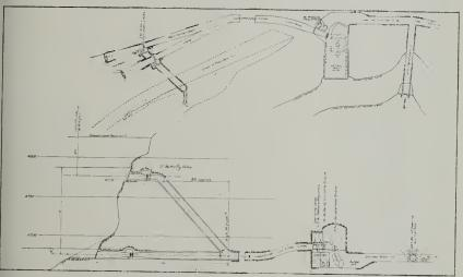
General plan and section of outlet works.
