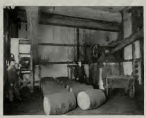
Grinding-room, showing a Williams grinder driven by a 50 h. p. motor.
